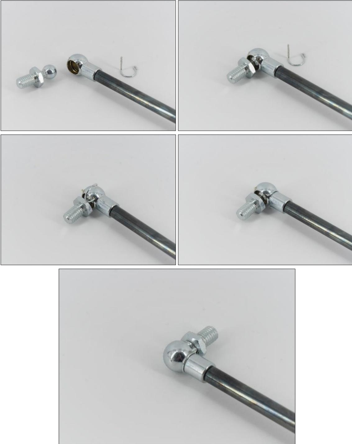
The safety retaining clip aids the retention of the ball stud in the socket housing, it must be removed before fitting or removing the ball stud from the socket housing.
